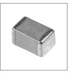
**CERAMIC CAPACITOR** This little guy is the same size as the resistors. Like the resistor, it has a metal cap on each end. It comes in various shades of tan, and it has no markings.
