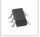
IC - SOT23 This one's called SOT23, which means Small Outline Transistor.
