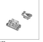
LED These little LEDs are pretty annoying! They're as small as the resistors and capacitors, and they have a polarity marking on the bottom, but no
